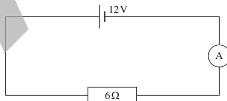
When the student changes the resistor in the circuit shown, the current changes from 0.02 A to 0.4 mA. What is the value of the new resistance? Was the information told to the student correct?
