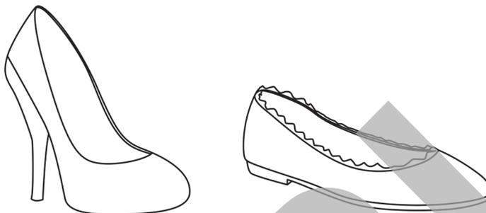
A woman whose weight is 600 N wears a pair of flat shoes. Each shoe has a surface area of 250 cm<sup>2</sup> in contact with the ground. What pressure does she exert on the ground? She then changes into stiletto shoes that both have a contact surface area of 75 cm<sup>2</sup>. What is the new pressure?
